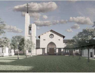
New Construction of a 24,000 SF Sanctuary, which includes a mezzanine and undercroft. Project shall consist of custom Precast columns, arches and walls, custom interior plaster veneer, custom Wassau glass and stained glass, air cooled chiller system, and exterior buff stone veneer cladding.
